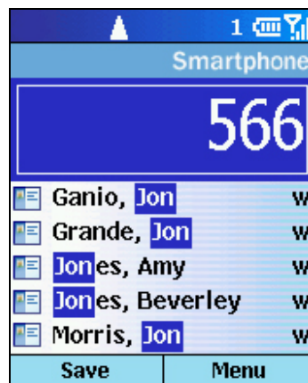
Figure 2. Smartdial displays a short list of contacts based on the letters you press.
