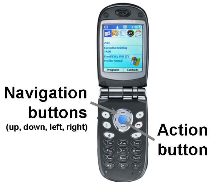
Figure 3. Navigation and Action buttons make it easy to move around the screen and make selections.
