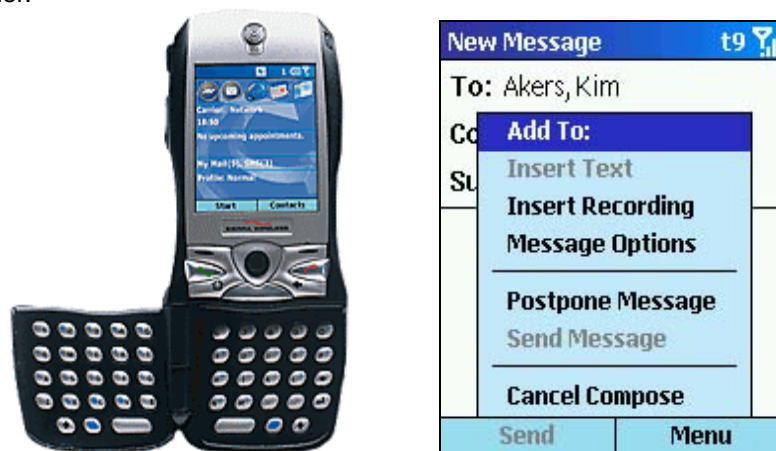
Figure 4. Either the built-in keyboard in Sierra Wireless' Voq Smartphone or the built-in voice recorder offers quick options for responding to e-mail.
